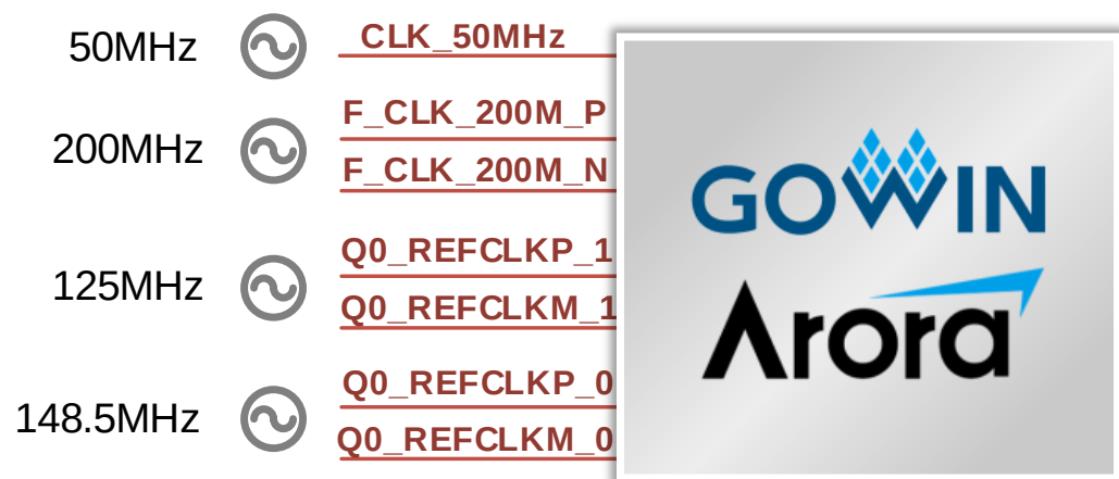
Figure 3-3 Clock Connection Diagram
