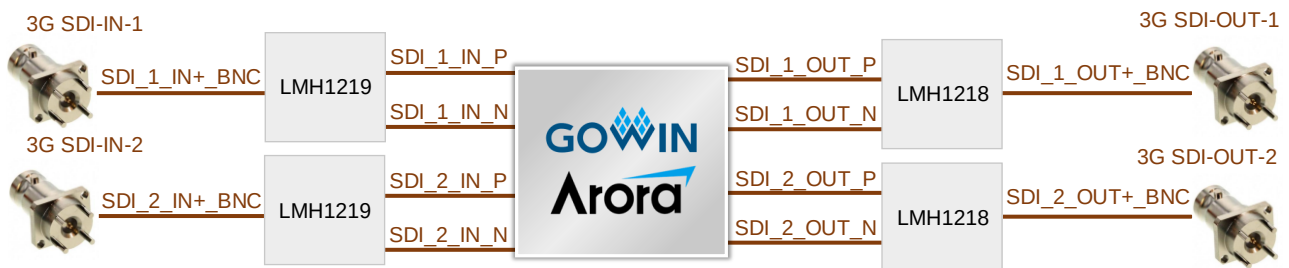
Figure 3-9 Connection Diagram of SDI Interface
