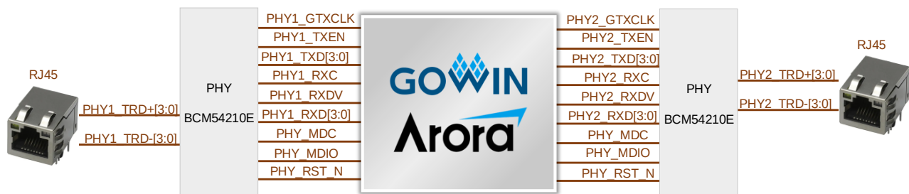
Figure 3-10 Ethernet Interface Connection Diagram
