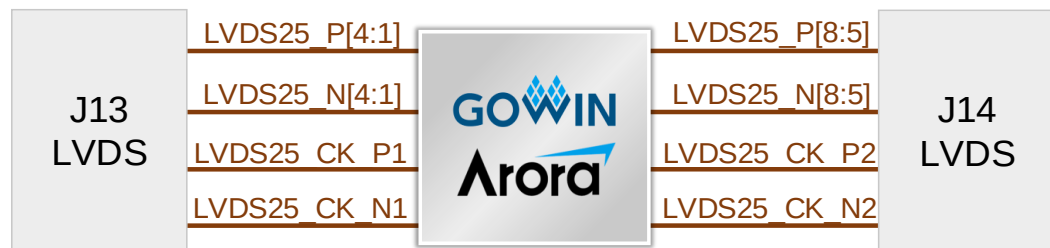
Figure 3-12 Connection Diagram of LVDS Interface
