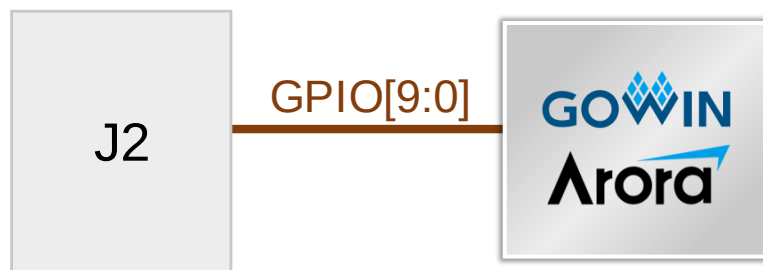
Figure 3-17 Connection Diagram of GPIO Interface
